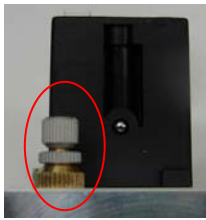
Continuous/Pulse change needle: ON (Continuous blow) OFF (Pulse blow)
