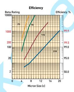
Notes: Multipass test run @ 80 l/pm to 3.5 bar terminal - 5 mg/l BUGL.
