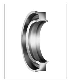
The profile design of the profile EM rod seal/wiper combines the profile geometry of our tried and proven profile EL with the requirements of mini-pneumatics, i.e. the dimensions of profile EM are considerably smaller and friction values are even lower.
